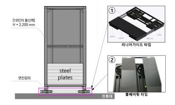
Fig. 1 Shake table testing of a communication rack with two types of base isolators
